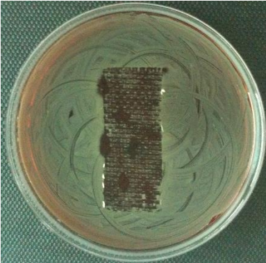
Figure 1. The antibacterial activities against Staphylococcus aureus (ATCC 6538) according to test method AATCC 147
